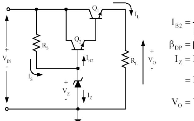
$$\begin{split} I_{B2} &= \frac{I_{E1}}{\beta_{DP}} = \frac{I_{L}}{\beta_{DP}} \\ \beta_{DP} &= \beta_1 + \beta_2 + \beta_1 \beta_2 \\ I_{Z} &= I_{S} - I_{B2} \\ &= I_{S} - \frac{I_{L}}{\beta_{DP}} \\ V_{O} &= V_{Z} - 2V_{BE} \end{split}$$
