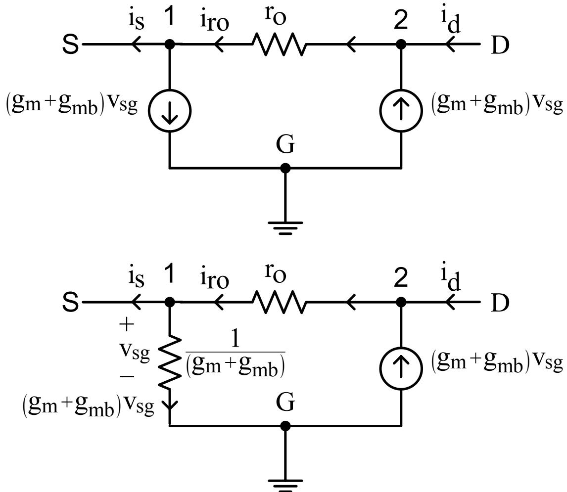
If  $r_o$  is finite, the circuit is bilateral because of the feedback. If  $r_o \rightarrow \infty$ , the cct. is unilateral.
