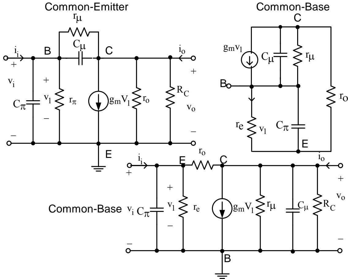
$C_\mu$  is between B-C. At high freqs., capacitive components are dominant.
