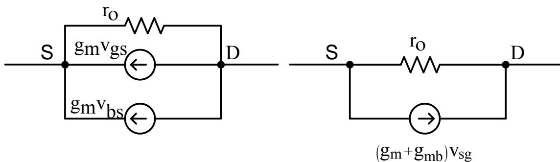
The body (B) is ac gnd,  $v_{bs} = v_{gs}$  because G is also at gnd.
