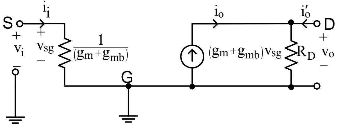
$$G_m = \left. \frac{i_o}{v_i} \right|_{v_o=0} = \frac{(g_m + g_{mb})v_{sg}}{v_{sg}} = g_m + g_{mb}$$
