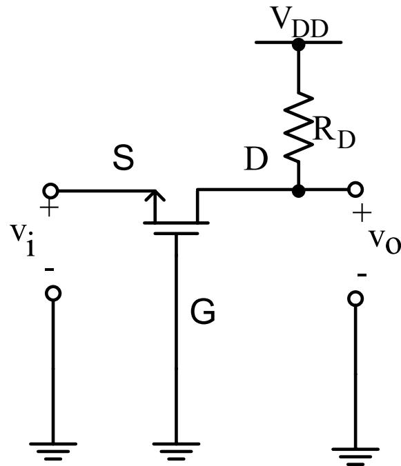
I/p signal is applied to the S. O/p is taken from the D. G is connected to the ac gnd.
