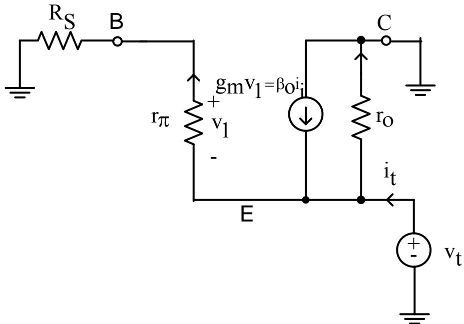
$$v_1 = -\frac{r_\pi}{R_S + r_\pi} (v_t)$$
