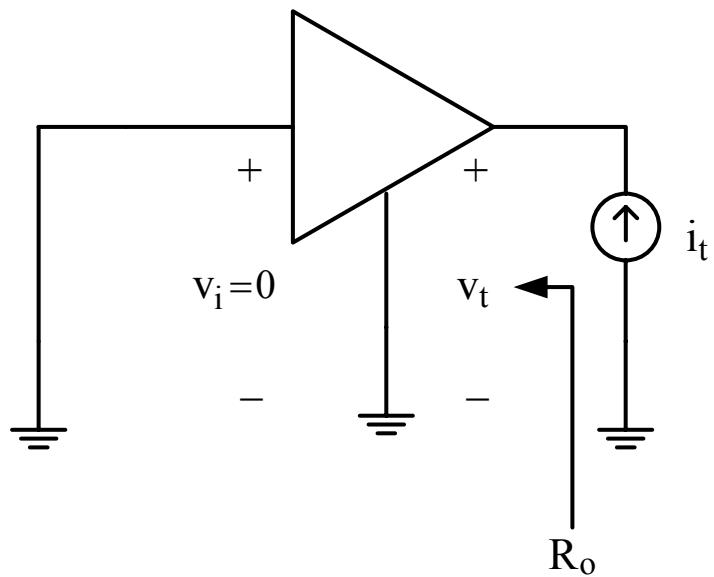
11. Output resistance of the amplifier proper
