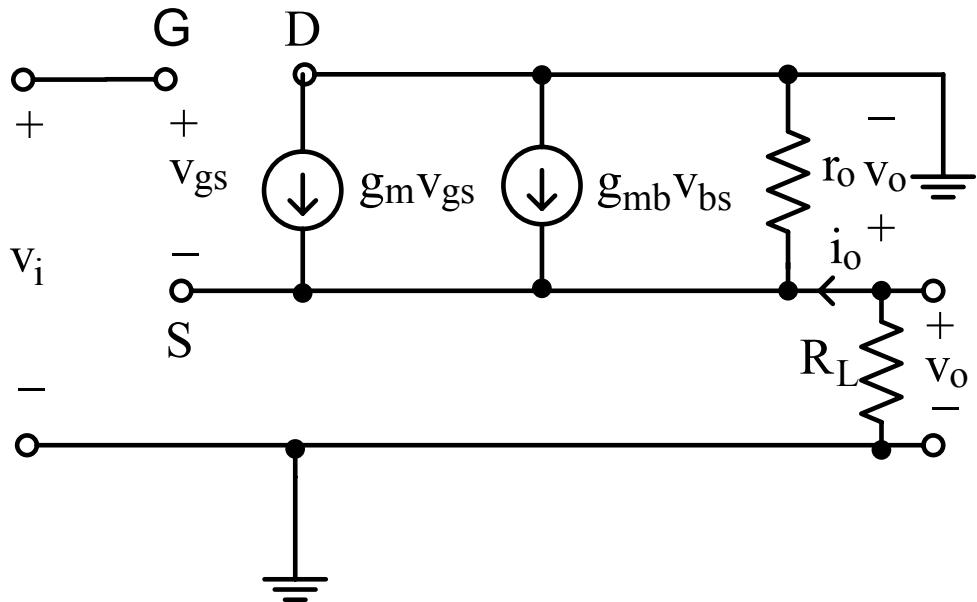
The output resistance can be calculated by setting  $v_i = 0$  and driving the output with a voltage source  $v_t$ .
