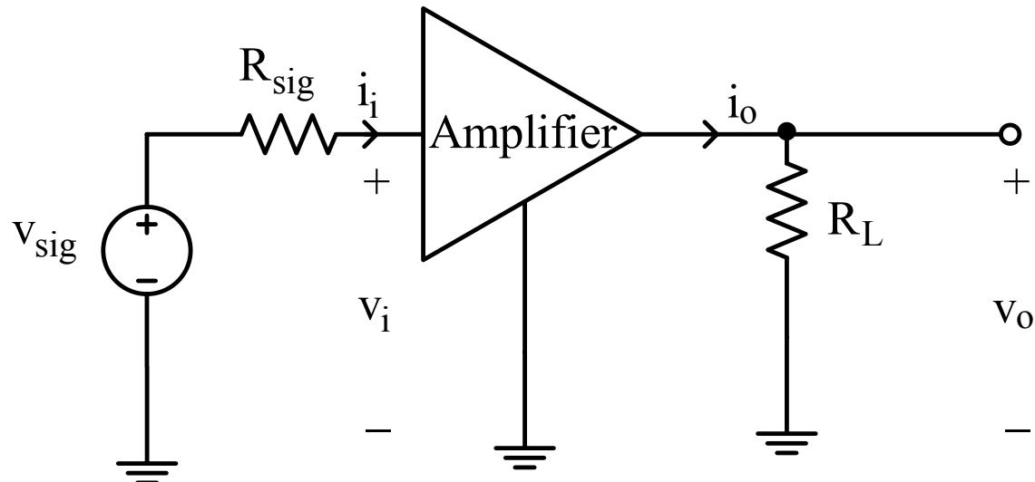
3. Open-circuit voltage gain
