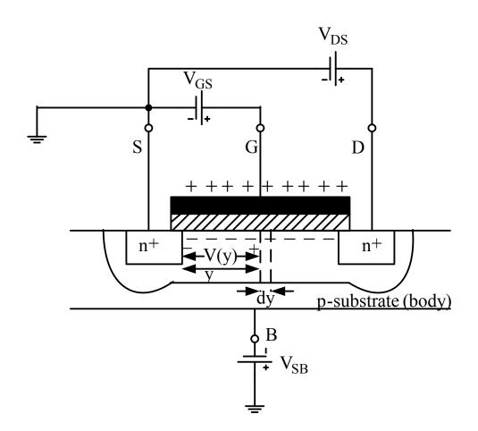
$\begin{array}{ll} Q_1(y) = C_{ox} \left[ V_{GS} - V(y) - V_t \right] & (1.145) \\ V(y) = \text{voltage at a distance y along the channel} \\ & \text{wrt S} \\ V_{GS} - V(y) = G \text{ to channel voltage at point y} \\ & \text{from S} \end{array}$
