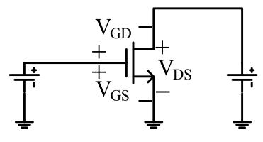
KVL around the transistor:  $-V_{GS} + V_{GD} + V_{DS} = 0$   $V_{DS} = V_{GS} - V_{GD} = V_{DG} + V_{GS}$ When  $V_{DS} > V_{GS} - V_t$ ,  $V_{DG} + V_{GS} > V_{GS} - V_t$ . Hence,  $V_{GD} < V_t$ . The channel no longer exists at D. At the point
