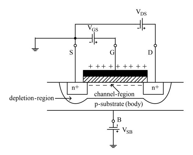
If  $V_{GS} > V_t$ , inversion occurs and a conducting channel exists. The channel conductivity is determined by the vertical electric field, which is controlled by the value  $V_{GS} - V_t$ . If  $V_{DS} = 0$ ,  $I_D$ = 0 because the horizontal electric field is 0. The value of the current depends on both the horizontal and the vertical electric fields, explaining the term field-effect transistor. +ve  $V_{DS}$  causes the rb from the D to the substrate to be larger than the S to the substrate.
