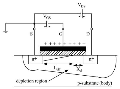
Increasing  $V_{DS}$  will increase the width of the depletion region around the D and reduces the effective channel length of the device in the saturation or active region. This effect is the channel length modulation and causes  $I_D$  to increase when  $V_{DS}$  is increased.
