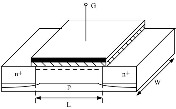
$C_{ox}$  = oxide capacitance per unit area from G to channel
