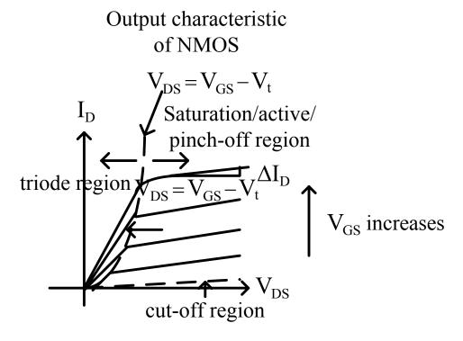
$V_{DS} > V_{GS} - V_t \rightarrow \text{pinch off / saturation region.}$  In saturation region, output characteristics are almost flat.  $I_D$  depends mostly on  $V_{GS}$  and only to a small extent on  $V_{DS}$ .
