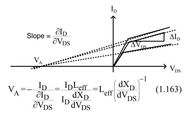
For MOSFETs, a commonly used parameter for the characterization of channel length modulation is:
