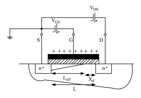
$$\Delta I_{D} = \frac{\partial \overline{I_{D}}}{\partial V_{DS}} \Delta V_{DS}$$
