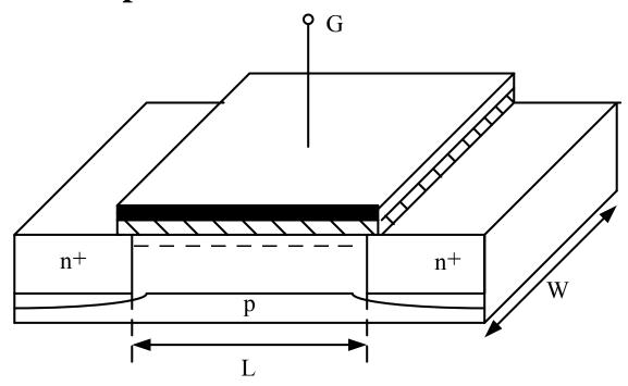
G is insulated from the channel by the  $SiO_2$ . At low-frequencies, G current is essentially 0 and input resistance is essentially  $\infty$ .
