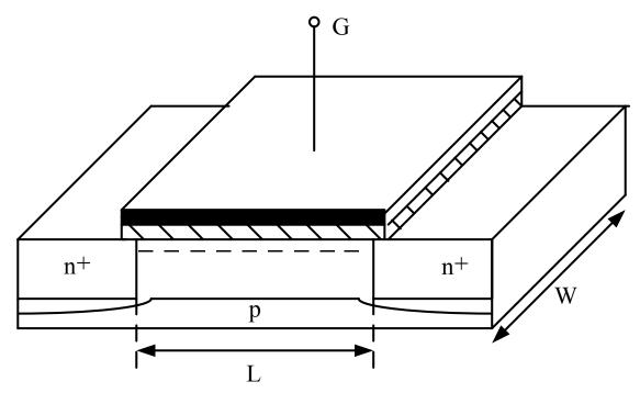
In the <u>triode region</u> of device operation, the channel exists continuously from S to D. The G-channel capacitance is usually lumped into two equal parts at the D and S,
