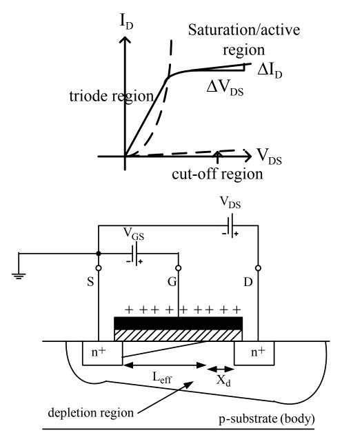
$X_d$  = depletion layer width between physical pinch-off point in the channel at the D-end and the D region itself.
