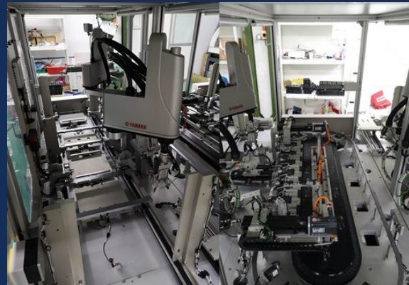
Scara Robot with Conveyor & Magnetic Linear Motors
